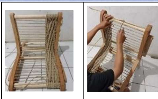
Figure 12. Weaving of Pandan fibers in a chair construction
